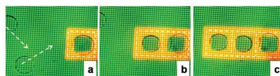
**Fig 2. Trapping of thermo-sensitive microgels with Ph-OET.** Square optical patterns were used to trap microgel particles. The applied voltage is 10Vpp at 1MHz frequency.
