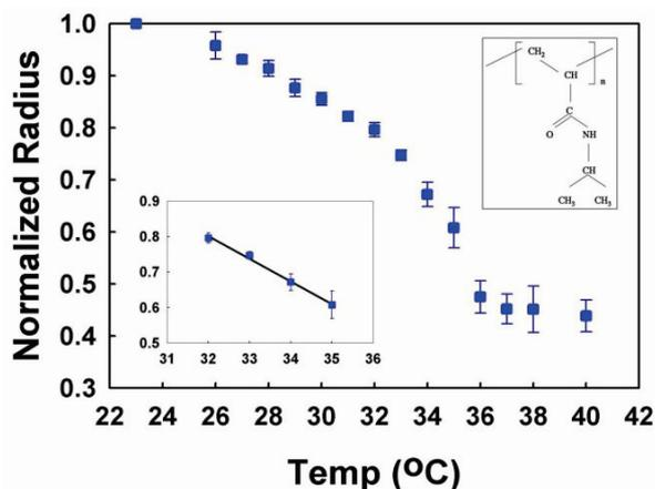
Fig 3. Radius of poly(N-isopropylacrylamide) microgels versus temperature. The radius is normalized to their size at 23°C.
