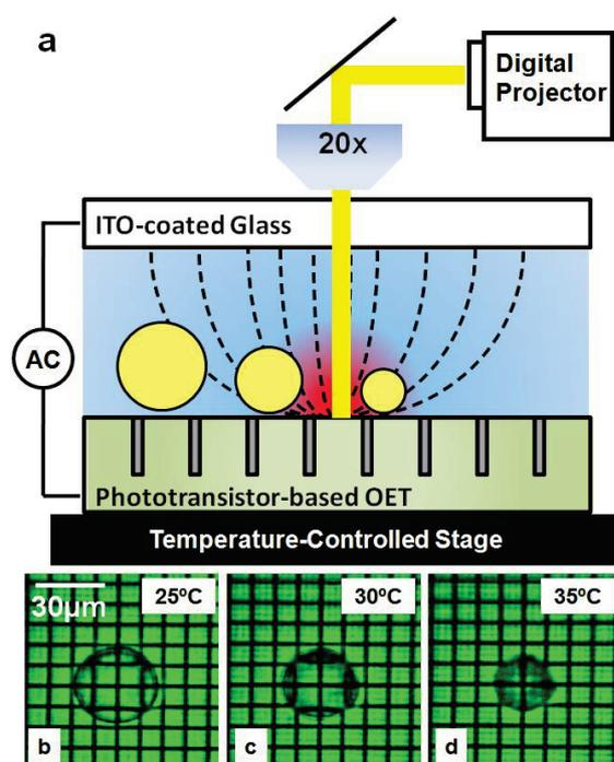
**Fig 1. (a) Schematic of Ph-OET device and the experimental set-up.** The light pattern activates the phototransistors and induces a local electric field. The thermo-sensitive microgels in the media respond to temperature rise by shrinking **(b-d) Images of Thermo-sensitive microgel at various temperatures.** As temperature increase, the microgels shrink in size.
