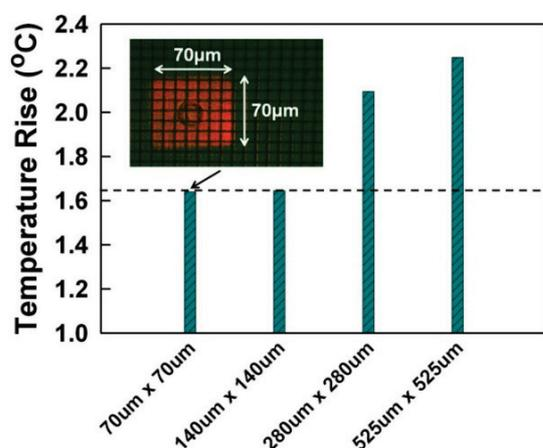
Fig 6. Measured temperature rise with square pattern of various sizes under  $20V_{pp}$  voltage bias. The dotted line shows the temperature rise without illumination.
