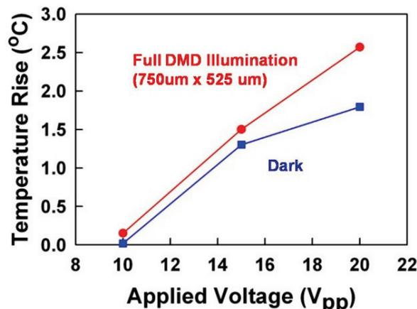
Fig 5. Temperature rise vs. electrical bias with and without illumination. The applied voltage was 20V<sub>pp</sub> at 1MHz.
