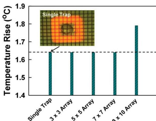
Fig 7. Measured temperature rise with different numbers of single particle trap under  $20V_{pp}$  bias voltage. The dotted line shows the temperature rise without illumination.
