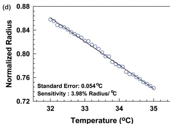
Fig 4. (a-c) Pattern matching process. (d) Normalized microgels radius as a function of temperature. The size of the microgel is measured with pattern matching.
